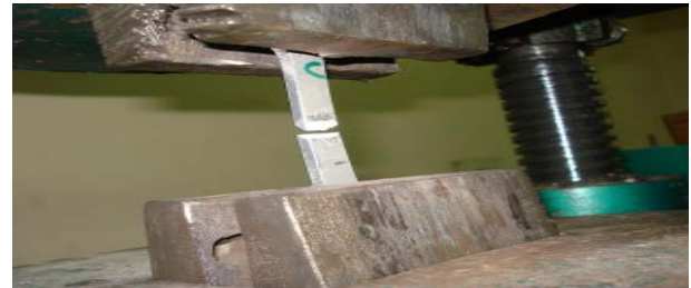
Figure 6 Schematic illustrations of tensile test specimens in the transverse direction to the weld zone.
